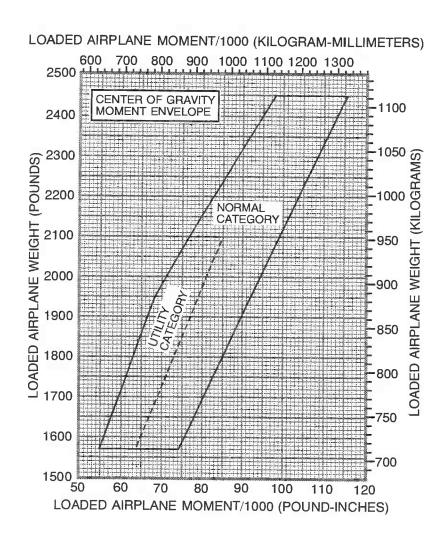
Figure 6-7. Center of Gravity Moment Envelope
