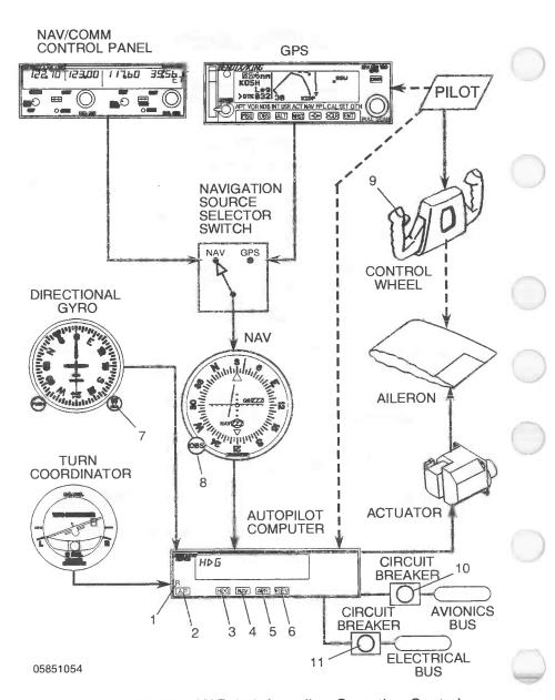
Figure 1. Bendix/King KAP 140 Autopilot, Operating Controls and Indicators (Sheet 1 of 2)
