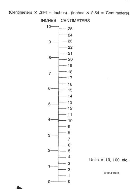
Figure 1-4. Length Conversions (Sheet 2 of 2)
