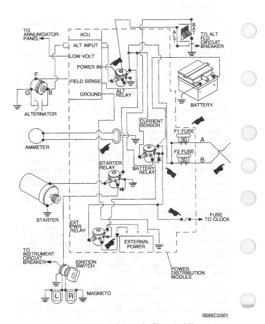
Figure 7-7. Electrical Schematic (Sheet 1 of 2)
