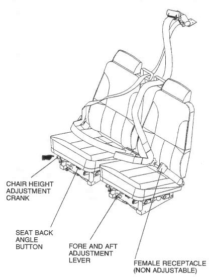
Figure 7-4. Seat Belts and Shoulder Harnesses
