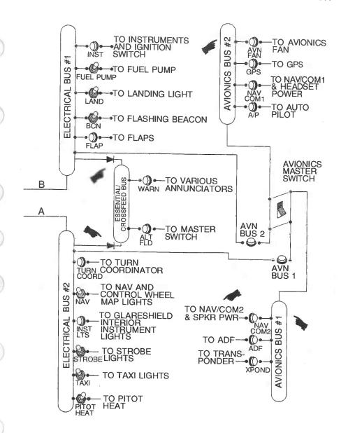
Figure 7-7. Electrical Schematic (Sheet 2 of 2)
